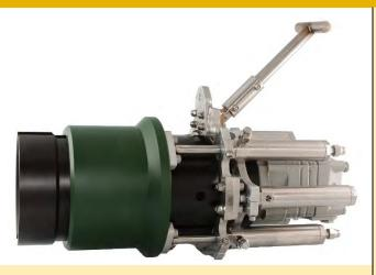
Cutting Head Diameter: Ø50 mm Feed Depth: 56 mm total System Pressure: 207 bar The TMT AM1 Valve Hole Cutting Tool is used to open subsea tree needle-valves that have deteriorated to the point where they can no longer be operated. This sometimes occurs during abandonment operations.
