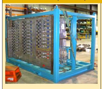
30 x lines @ 3500 psi 2 x lines @ 10000 psi 4 x accumulators The Intervention & Work Over Control System (IWOCS) skid is a self-contained High Pressure Unit (HPU) providing 30 independently controlled lines to 3000 psi and 2 lines to 10000 psi.
