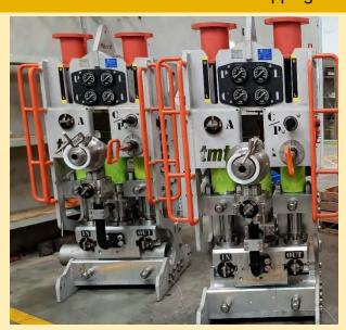
Tools that allow hot tapping into pressurised lines from ½" to 7" for flushing, dewatering, bleed-off, control, cementing. The tapping is done without introducing any swarf into the pipeline.
