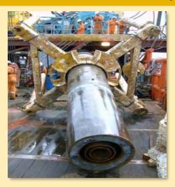
Casings: 7" to 36" Operating pressure: 14,000 psi The AXE system is used to sever multiple casing strings below the mud-line.
