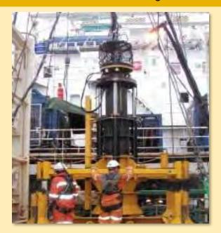
The TMT Subsea Top drive can retrieve both Internal Tree Caps and Tubing Hangers, which require a torque to be applied, normally via drill pipe from a rig. This tool was specially developed to assist in rigless abandonment of subsea wells.
