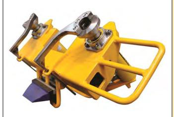
Max. Pressure: 700 bar (10,000 psi) Cylinder Stroke: 152 mm (6") Connector Stroke: 89 mm (3.5") The 4" Collet Connector Mechanical Override tool is used to actuate the collet when the hydraulic release mechanism has failed.
