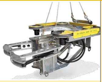
Diamond Wire Saws (DWS) are used to cut medium diameter structures. The tool clamps to the structure using the front mandibles. Then a moving abrasive wire is fed into the structure, removing material proportional to the applied speed and feed rate.
