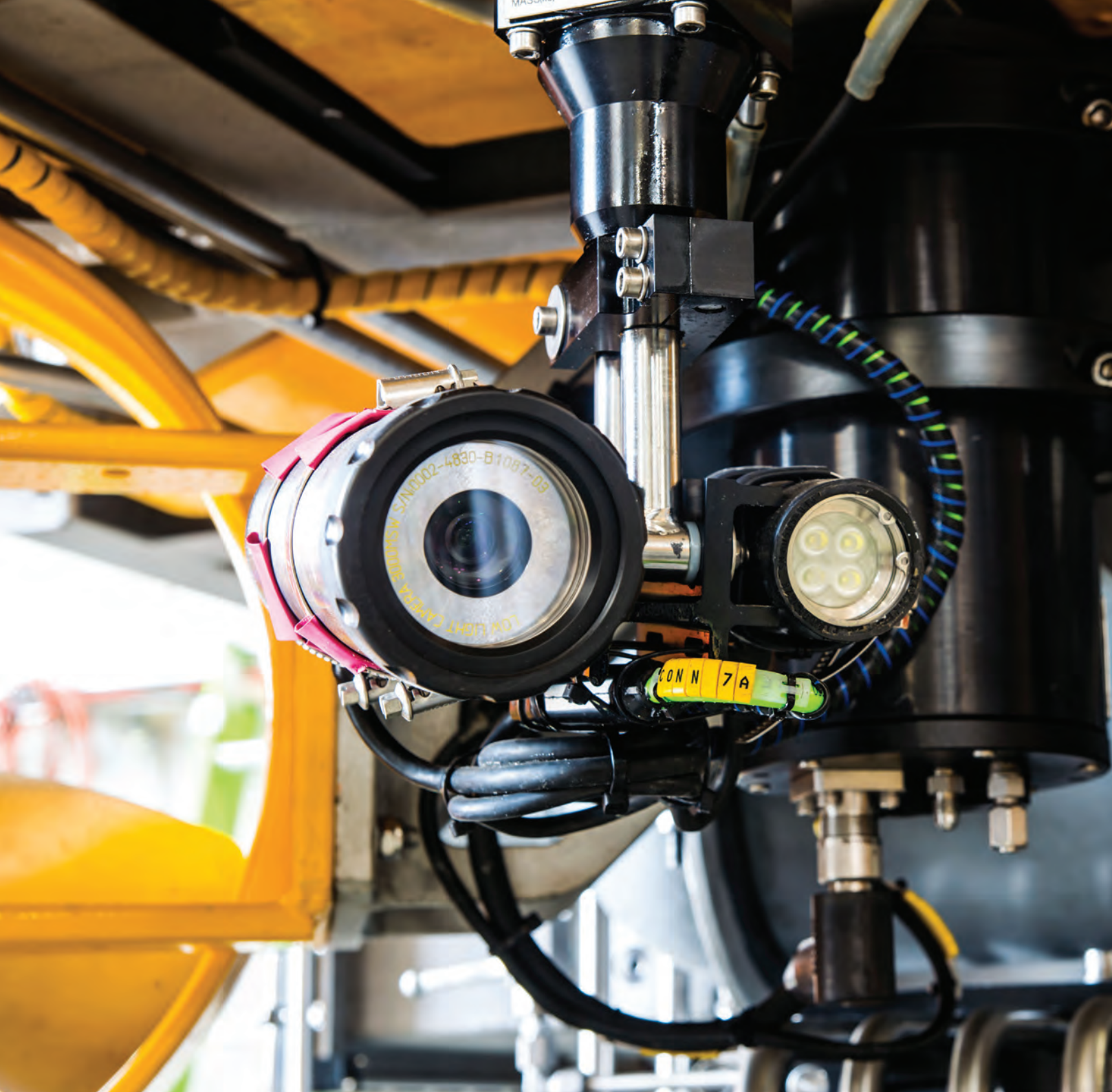
A TMT Low Light Camera combined with a TMT LED Light and installed on a Pan and Tilt module.
