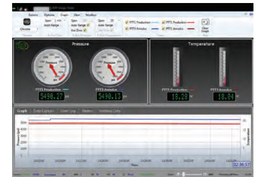
The interface for monitoring the TMT Gauge Tester.
