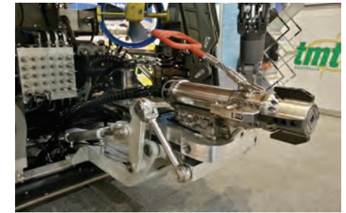
A TMT HD FLOT with a Smart Torque Tool operating from a Typhoon ROV.
