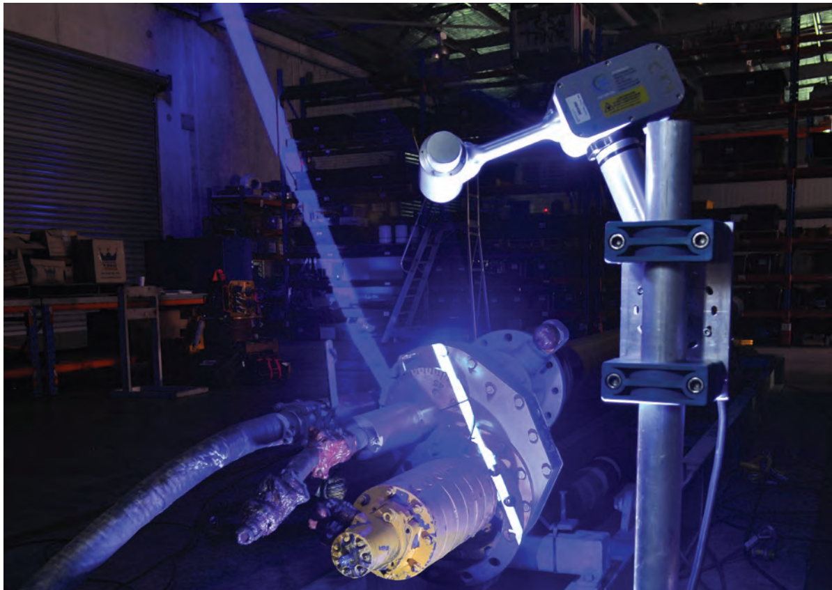
3D laser scanning using the 2G Robotics ULS-200.
