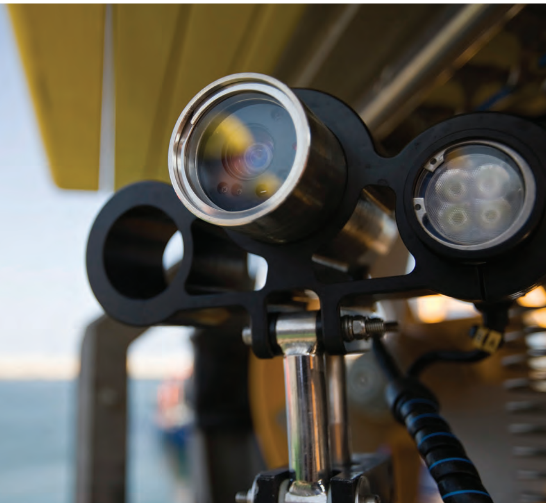
A TMT Colour Camera alongside an LED light mounted on a pan and tilt module.
