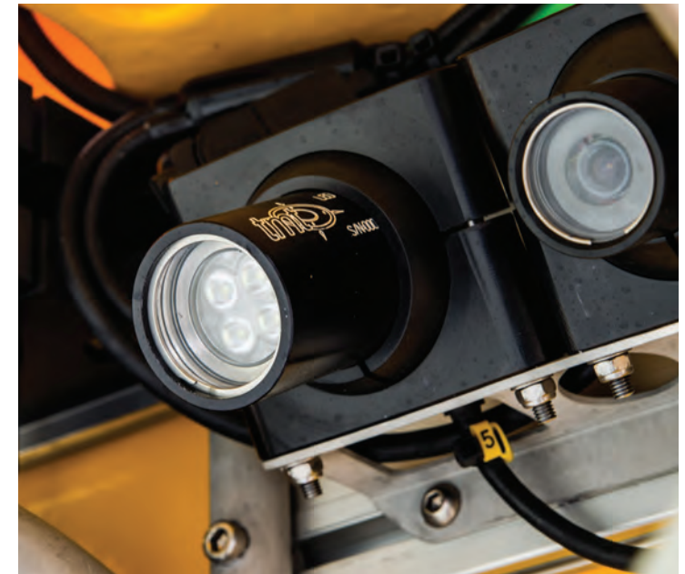
A TMT LED Light and camera in a fixed ROV mount.
