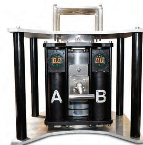
A TMT Smart Level mounted to a customised frame for use by an ROV.
